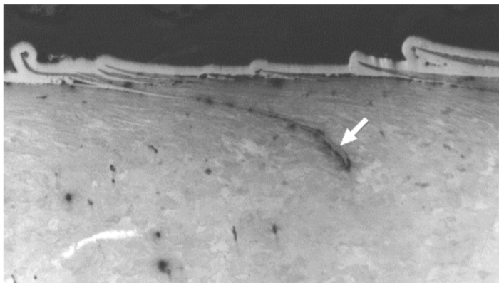
Figure 14.(c): Ratcheting Strains in Rail Material Caused by Large Longitudinal Creep Forces Between Wheel and Rail
